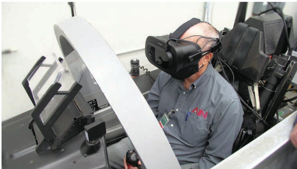
FlightSafety's T-6B trainer combines real controls with a simulated outside view in the headset.
