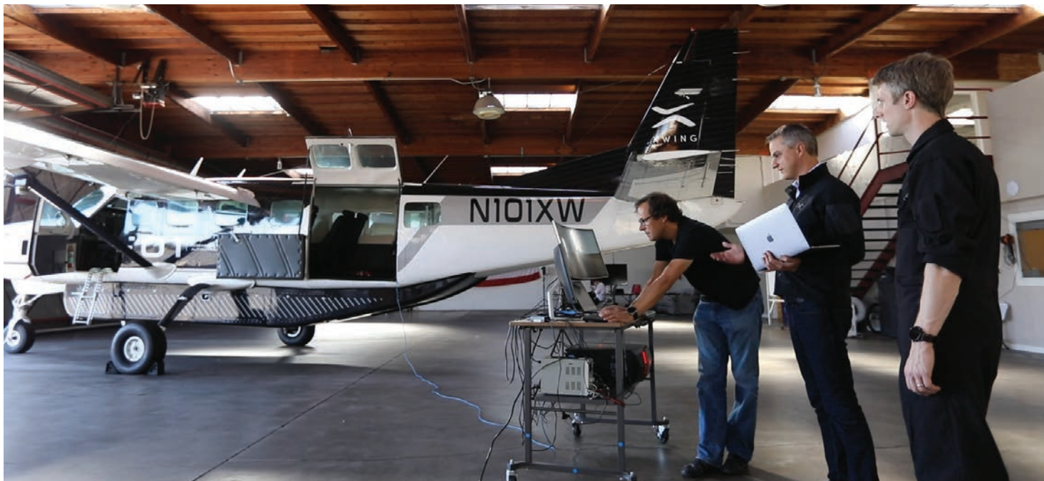
Xwing's autonomous flight system is undergoing testing in a Cessna Caravan single-engine turboprop.
