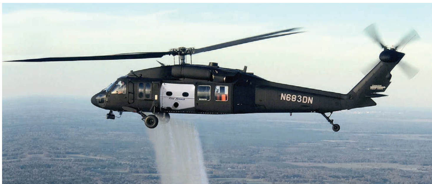
The Rogerson Kratos Top Drop conversion of the Black Hawk costs about one-third of the price of a new fire-fighting helicopter.
