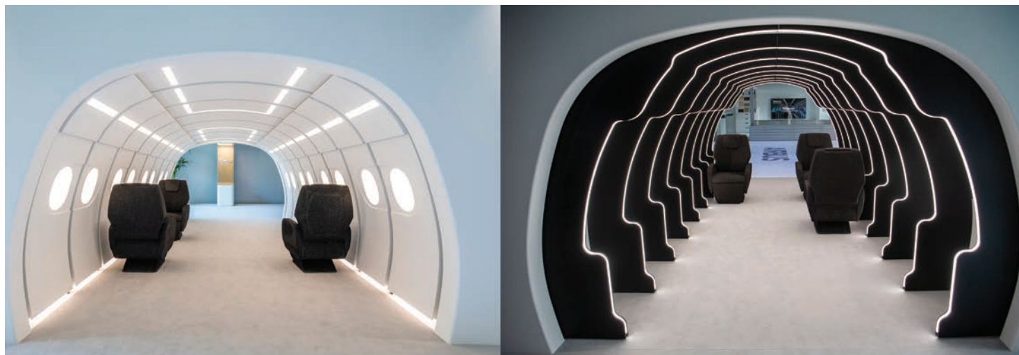
At the ACJ TwoTwenty creative studio, a full-size cabin mockup is fitted with retractable elements (right) that help illustrate the difference in size between the ACJ TwoTwenty's cabin and typical modern ultra-long-range business jets.
