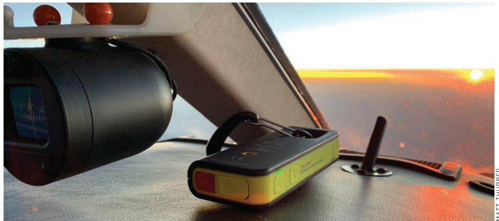
ACR Electronics' Bivy Stick Iridium satellite messaging device worked well at FL410 in a CitationJet.
