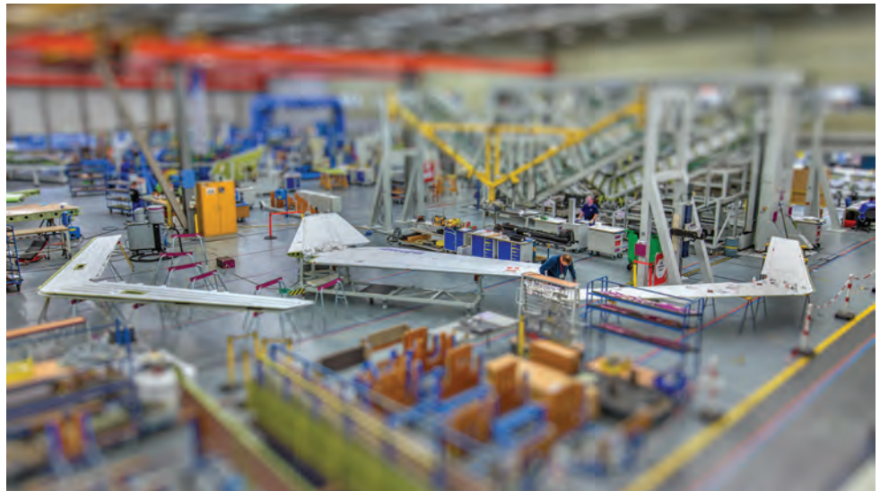
GKN manufactures empennages with thermoplastic rudders and elevators at its factory in Papendrecht, the Netherlands.
