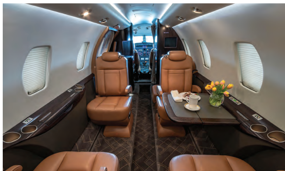
West Star Aviation’s Alton, Illinois, facility refurbished this Citation 560, with full soft goods replacement and sand stain over refinished matte wood.
