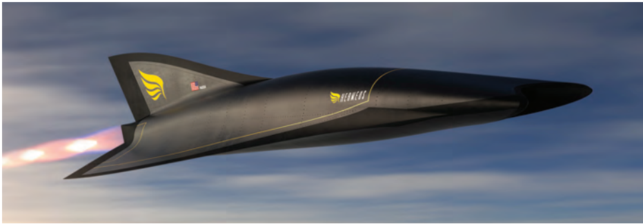
The small-scale Hermeus Quarterhorse will be flown autonomously and will be used for flight testing at speeds between Mach 3 and Mach 5.
