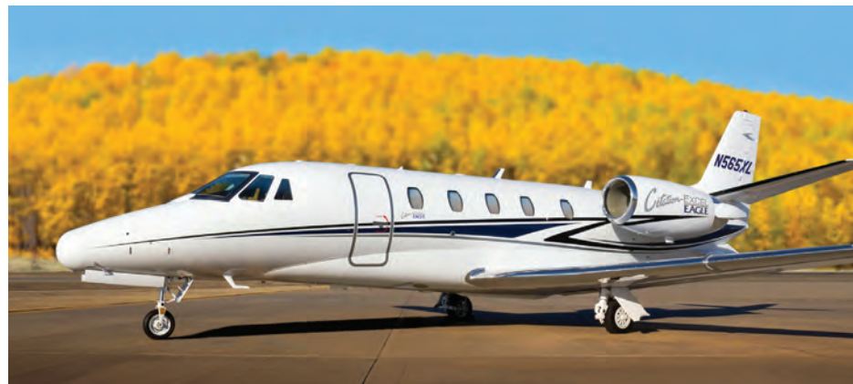
The refurbished Citation Excel Eagle program brings the popular business jet into the modern age with updated Garmin G5000 avionics, fresh paint and interior, and other improvements.
