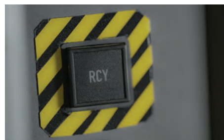
We flipped the Falcon 7X nearly upside down before pushing the recovery button.
