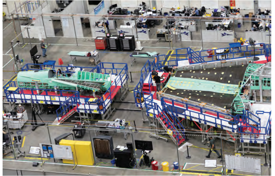
NASA declared the X-59 has reached the halfway mark in development, with the wing closed and fuselage and empennage ready to be joined.
