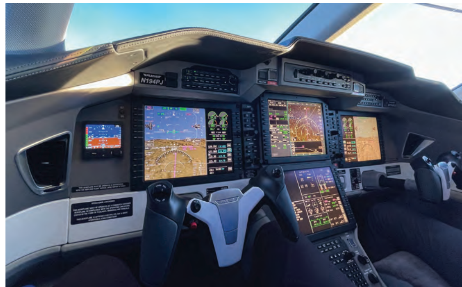
The PC-24 flight deck features a Honeywell Epic-based avionics suite, cursor-control device interface, and autothrottles.
