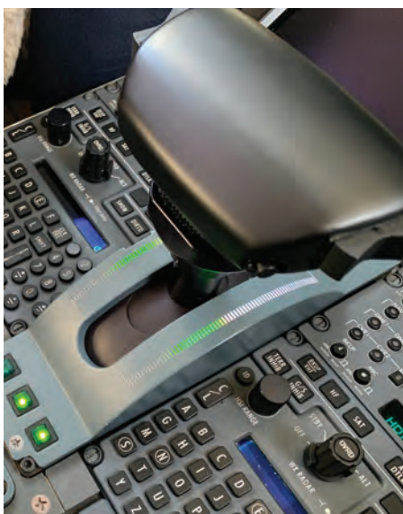
The flight test SmartThrottle has LED light strips on either side to highlight engine condition.
