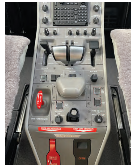
The PC-24 flight deck features a Honeywell Epic-based avionics suite, cursor-control device interface, and autothrottles.
