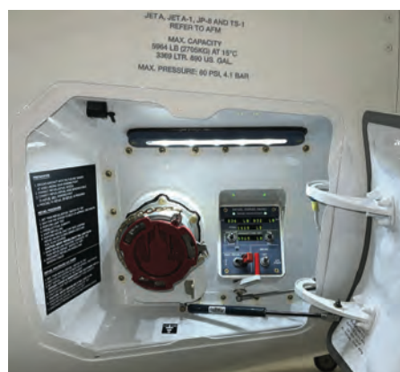
Single-point refueling is the quickest way to fill the PC-24 with a maximum load of 5,964 pounds of jet-A.
