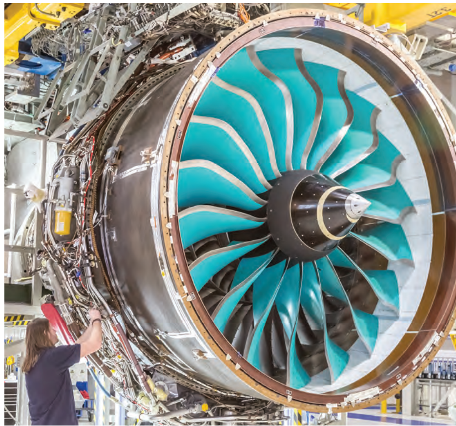
Rolls-Royce engineers in Derby, UK, prepare to test the UltraFan's composite fan system.
