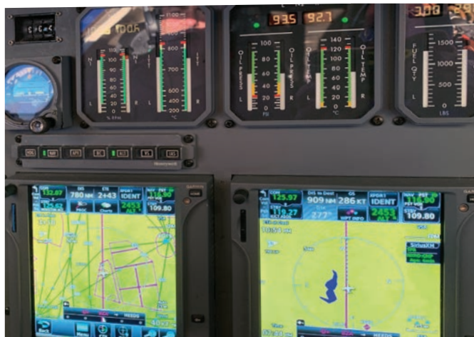
Leveling off at FL410 on the flight to San Diego in the Tamarack-modified CitationJet, burning just 300 pph per engine.
