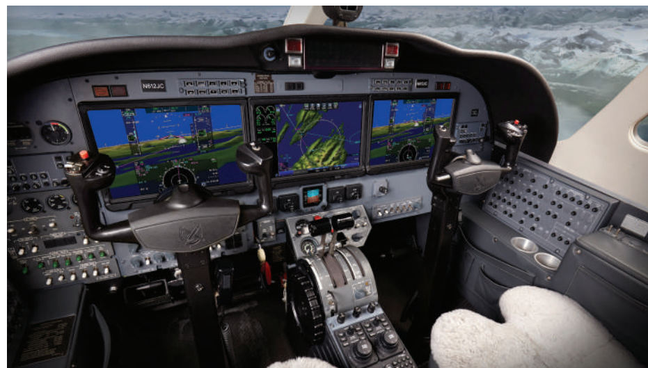
Collins Aerospace is certifying its Pro Line Fusion touchscreen integrated flight deck in the CJ2+ in April and will follow with STCs for the CJ1+ and CJ3.
