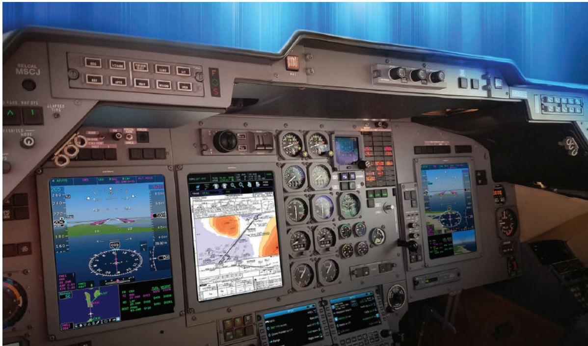
Universal Avionics' InSight flight deck for the Hawker 800XP includes three EFI-1040 displays.
