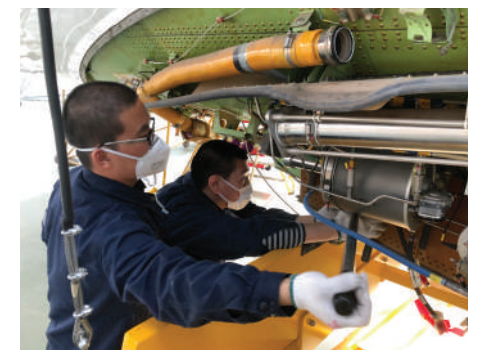
ExecuJet Haite's 96-month inspection of an Embraer Legacy 650 lasted eight weeks.
