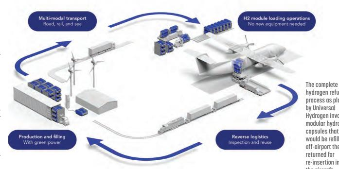
hydrogen refueling process as planned by Universal Hydrogen involves modular hydrogen capsules that would be refilled off-airport then returned for re-insertion into the aircraft.
