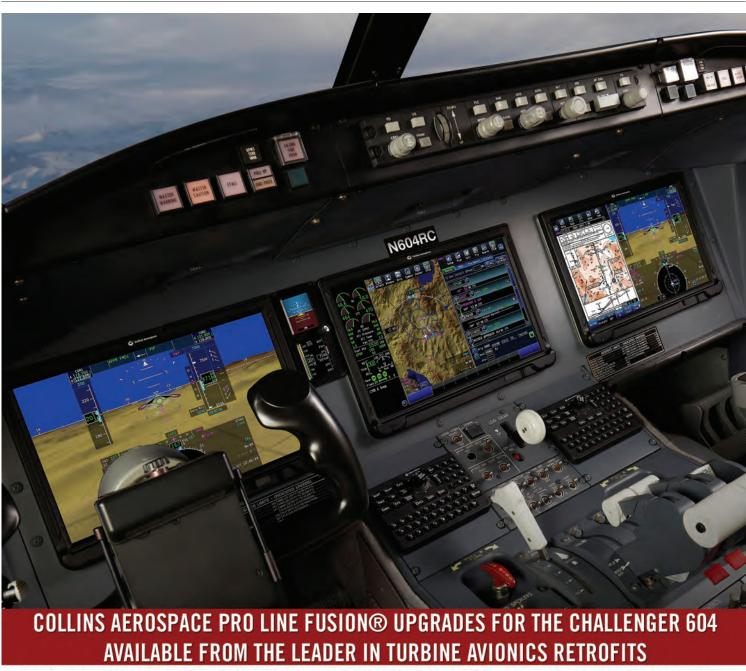
The Collins Aerospace Pro Line Fusion® upgrade for the Challenger 604 replaces the existing Pro Line 4<sup>TM</sup> avionics system with the latest touchscreen display technology. Standard features include synthetic vision, LPV/RNP approaches, and greatly improved FMS interaction and functionality. Some of the available optional upgrades include MultiScan<sup>TM</sup> weather radar, CPDLC, and FANS 1A.
