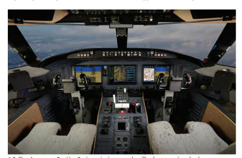
A Collins Aerospace Pro Line Fusion avionics upgrade will solve upcoming obsolescence issues facing Pro Line 4 displays and other key components on Bombardier Challenger 604s.
