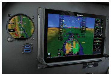
Garmin's GSB 15 chargers come with new features that include increased power output up to 27 watts per port and either dual Type-C or combined Type-C and Type A USB ports as well as short-circuit and over-temperature protection.
