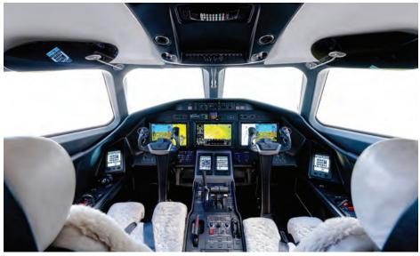
The Longitude's spacious flight deck features Garmin's G5000 avionics suite with four touchscreen controllers.
