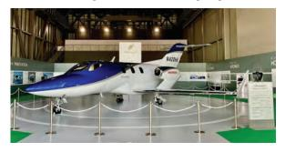
(OTWEM) design wasn't intended to make the Honda-Jet look unusual, which it certainly did, but took advantage of aerodynamic optimization that delays drag rise at high speeds. Although this was confirmed in a Boeing wind tunnel, the POC flight testing proved that the concept worked. Another key benefit of OTWEM is the larger space available in the cabin by moving engine structure and systems out of the fuselage.
