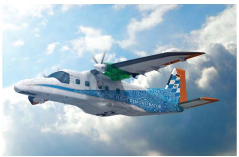
MTU Aero Engines is working with German aerospace research agency DLR to develop a technology demonstrator to power a Dornier 228 with hydrogen.
