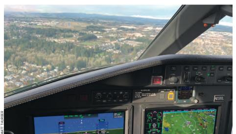
On final for the Runway 31L RNAV approach to KHIO with autothrottles and autopilot engaged, ready for the test of the coupled go-around capability.
