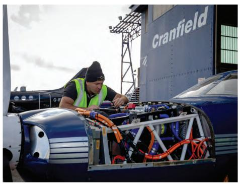
ZeroAvia's hydrogen propulsion system installed in a Piper M Series single-engine aircraft.
