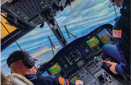
Honeywell's Phase 8 upgrade adds track-centered synthetic vision system and new offshore instrument approach capabilities to the Leonardo AW139.
