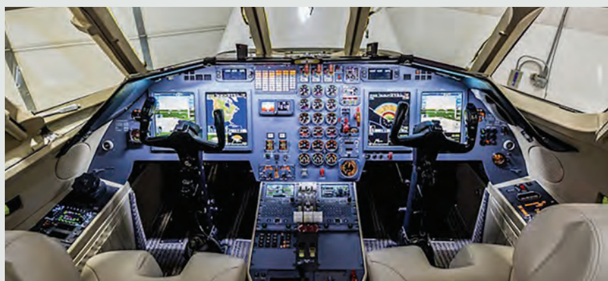
The Falcon 900B panel upgrade includes four Universal Avionics InSight displays, as well as touchscreen CDUs, alphanumeric keyboards, and a Mid-Continent standby module.
