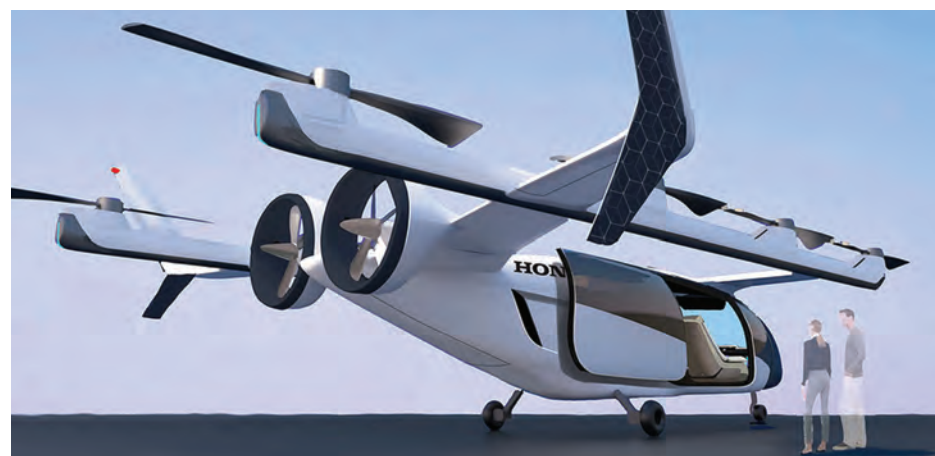
Honda said its eVTOL aircraft will provide a level of safety equivalent to that of commercial passenger airplanes, thanks to a simple structure and decentralized propulsion system.
