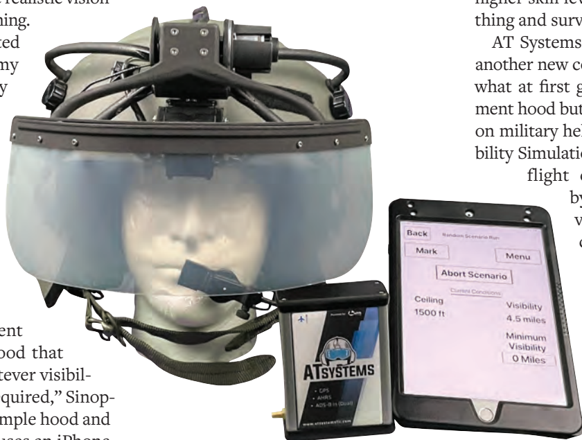
The AT Systems Visibility Simulation System helps helicopter pilots adapt to weather, dust, and other visual hazards.
