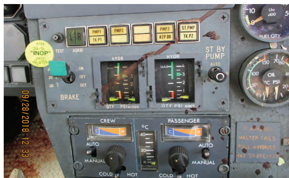
Among the many discrepancies that rendered the Falcon unairworthy, the brakes barely worked with the switch as shown, and worked better but without anti-skid in the other positions.
