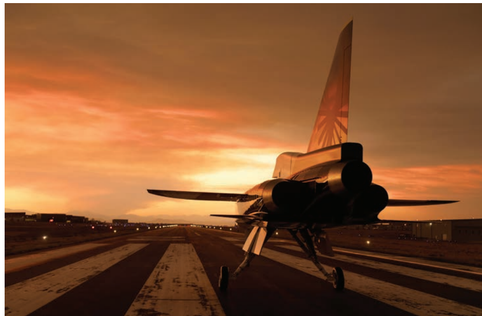
Boom Supersonic recently rolled out its XB-1 third-scale demonstrator, which is designed to explore technologies applicable to the company’s Overture supersonic airliner.
