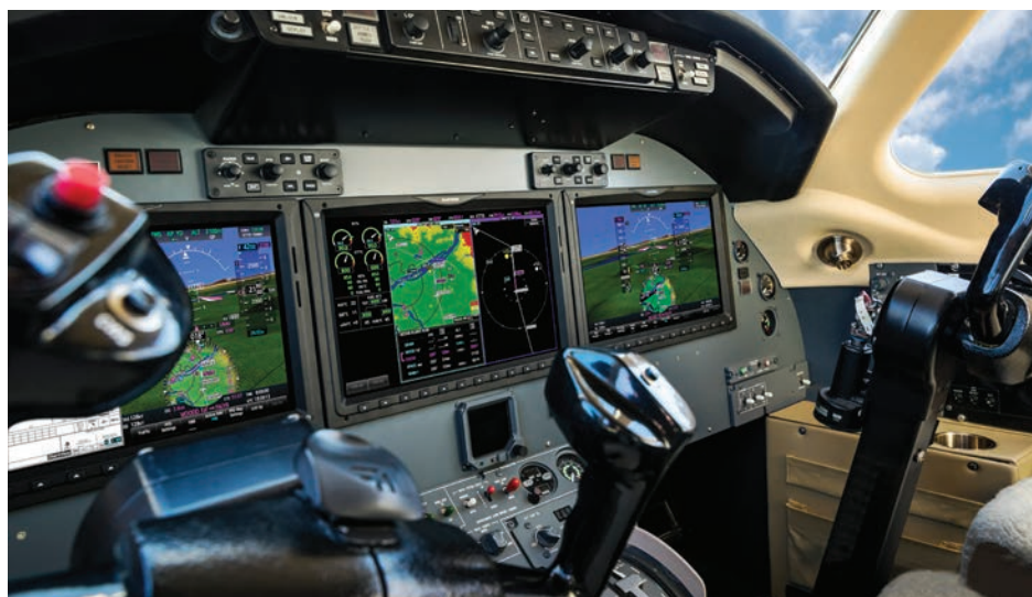
Even older jets like this Citation Excel can be upgraded with the latest Garmin G5000 avionics so pilots can take advantage of modern technology benefits.
