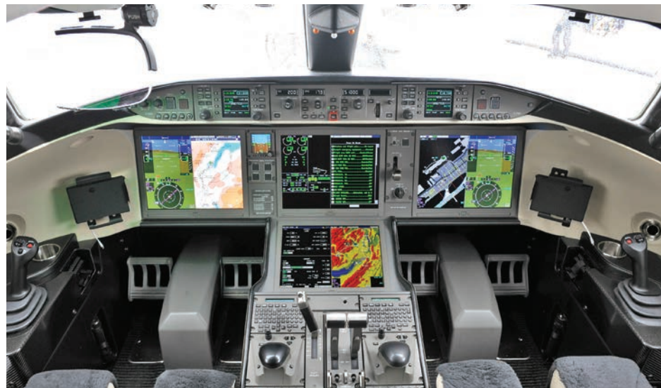
Bombardier’s Global 7500 features fly-by-wire flight controls and the Vision flight deck with the latest Collins Aerospace Pro Line Fusion-based avionics.
