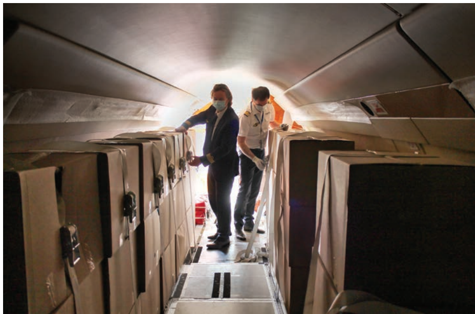
Dassault converted this Falcon 900B and a Falcon 8X to cargo configuration to carry medical supplies and doctors to small airports in France to help battle the coronavirus.
